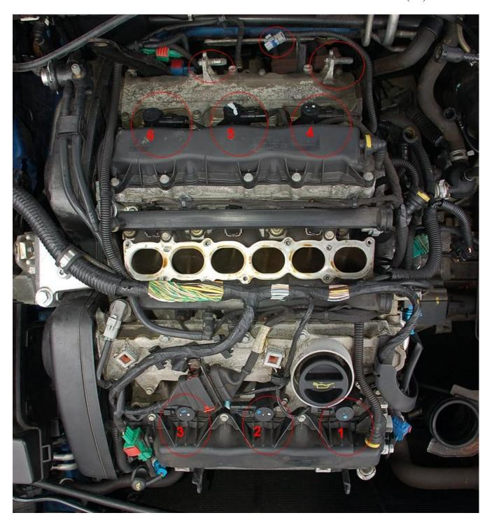
Remove the coil electrical connection (circled). A single 8mm bolt (circled) holds each coil in position. remove the bolt and the coil should wiggle out easily.
