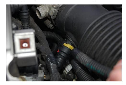
8. **Remove the brake servo pipe (K)** - Another of these union fittings like the breather hose. press in the bit on the back and it slides off easily
