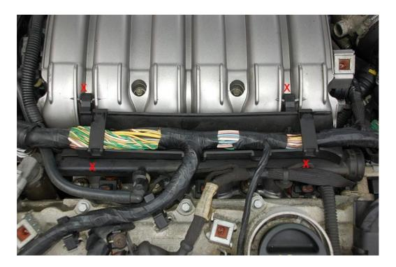
Just unclip the clips marked with an X and pull out from under the harness. Some parts of the harness are clipped on to the front of the engine, unclip these too if you need more slack on the wires
