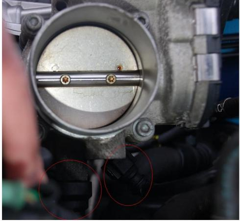
10. **Remove the wiring harness trunking -** This has to be removed in order to get to the bolts securing the intake manifold.
