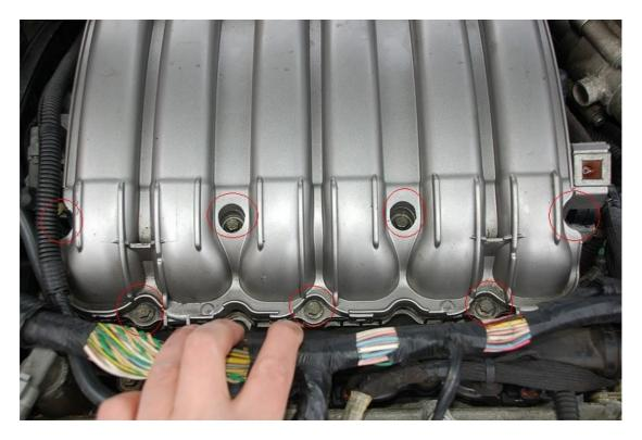
Take out all 7 bolts (take note of the 2 longer ones that should go back in the rear centre). Lift the manifold up at the front and then slide to the right to release from the rear mountings. Put the manifold somewhere clean while you carry out the rest of the work. Avoid touching the throttle butterfly valve or getting any dirt into the intake runners. Take care not to drop anything down the now fully exposed engine intake channels.
